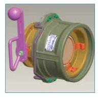
Fully rotate the operating handle to close the coupler. Grasp the bail on the operating handle and the recock handle assembly and move the recock handle towards you until the sleeve is fully retracted and locked.
