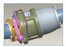
Connect the coupler to the adapter. The sleeve will slide completely, fully forward. Fully rotate the operating handle and in the open position, the operating handle cam surface should prevent the sleeve from sliding back.
