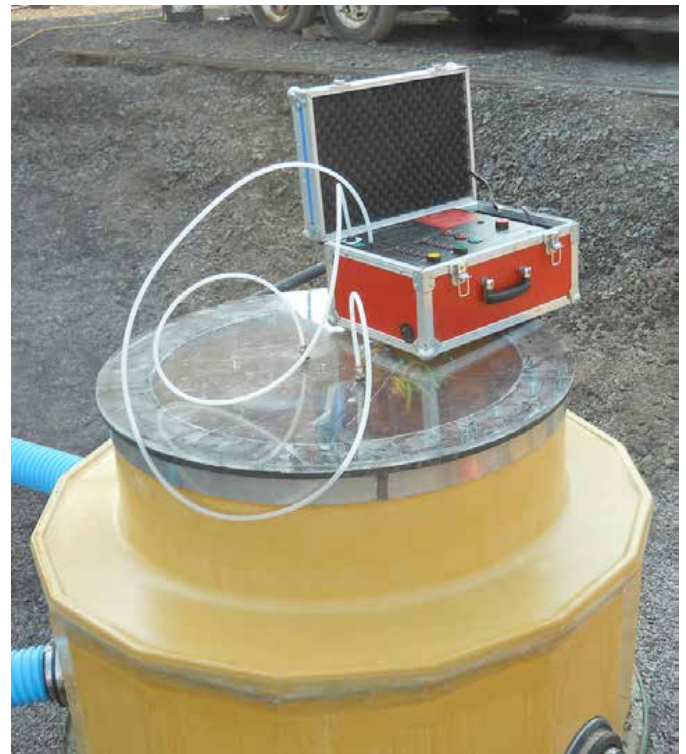
Vacuum testing to ensure a watertight installation
