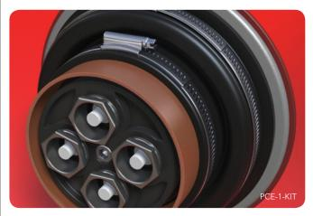
Fibrelite's range of pipe and cable entry kits offer a unique design allowing a single hole installation. No additional screw holes need to be drilled. This provides the installer with a quick and easy installation and minimises potential leak paths through the sump wall. The pipe sleeves are made from a fuel resistant nitrile grade or viton rubber and the bellowed design facilitates movement with changing ground conditions.
