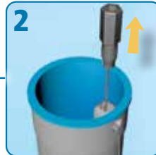
Lift float with cable to simulate fill
