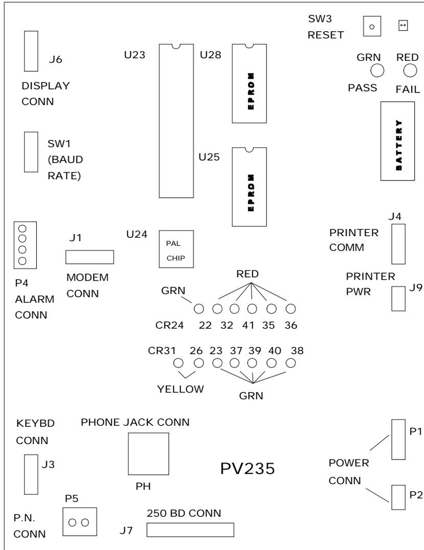
Figure H1 - CONTROLLER BOARD (PV235)
