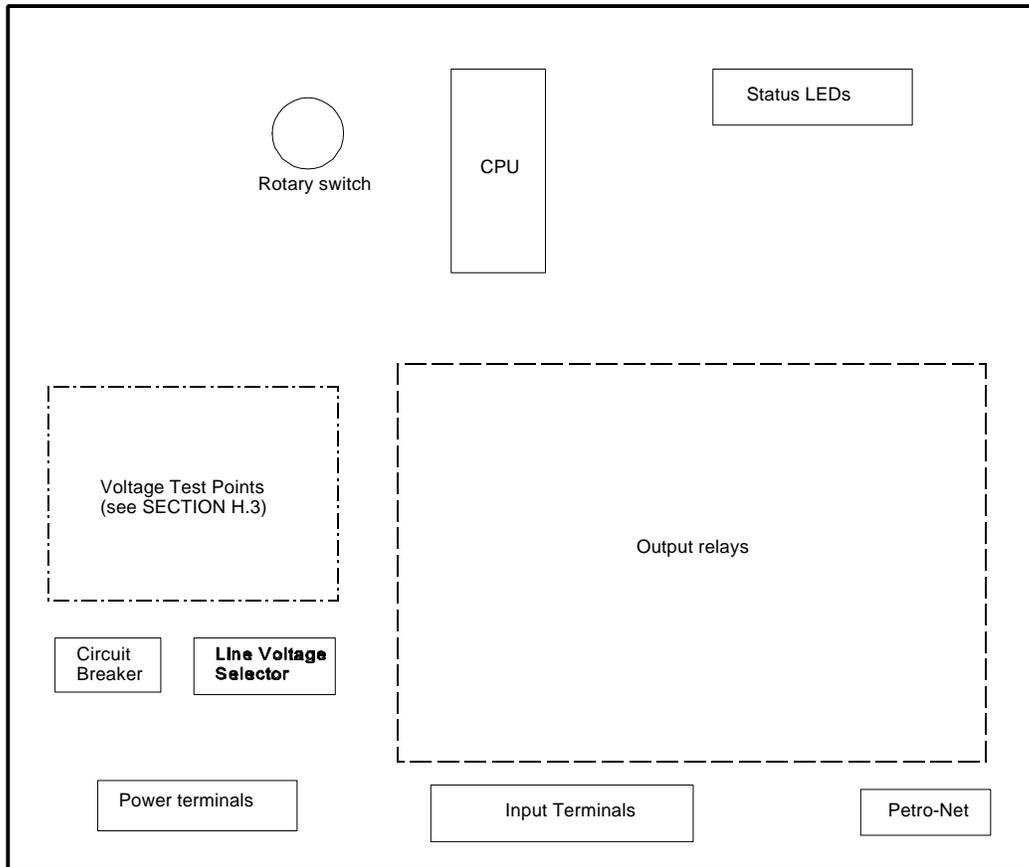
Figure H4 - I/O MODULE BOARD COMPONENT LOCATION
