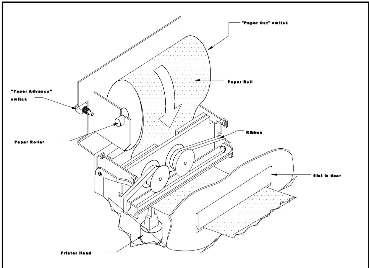
Figure I-1 - PRINTER PAPER REPLACEMENT
