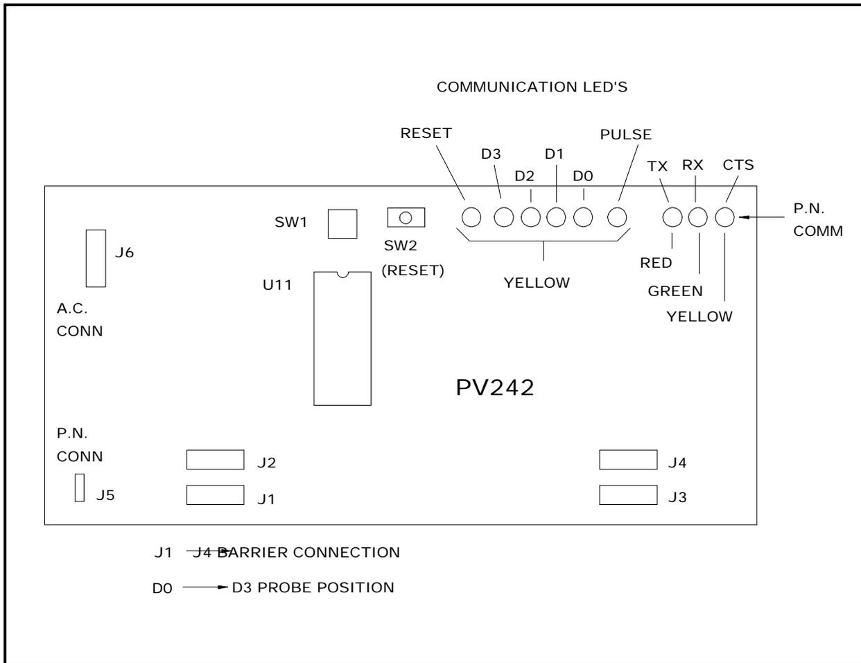
Figure H3 - SMART MODULE BOARD (PV242)
