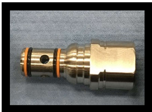
Figure 4. Breakaway Module with O-rings and backup rings
