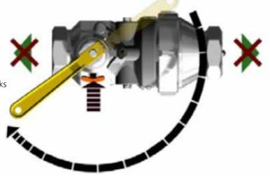
8. To disconnect the system, press the safety release button on the coupler and turn the handle clockwise so that it is parallel with the coupler. Press down on the clamp's tab (opposite side of safety release button) and push down on the handle to disengage the system
