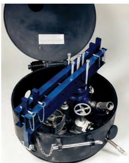
A typical ERK consists of a toolbox containing tools and replacement parts, as well as a bridge that is used to secure a cover can to the railcar's man-way cover plate.
