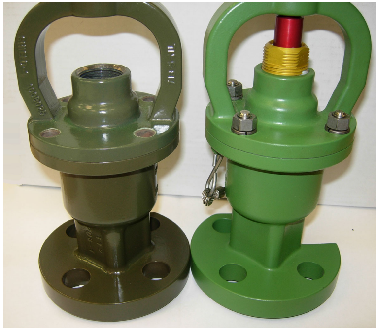
Figure 1: New ECTFE Coating (on left); Current ECTE Coating (on right).
