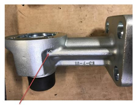
View of over drilled hole on 18-4-CS
