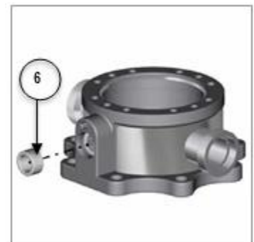
Figure 3-6 Remove Stop Plate and Stem
