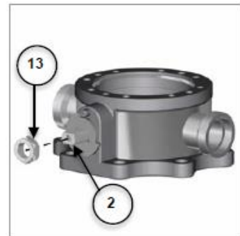
Figure 3-4 Remove Valve Ball
