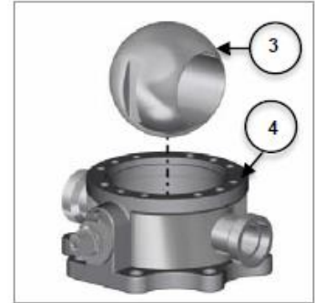
Figure 3-4 Remove Valve Ball
