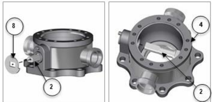
Figure 3-6 Remove Stop Plate and Stem
