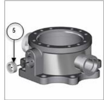
Figure 3-8 Remove Teflon ® Packing
