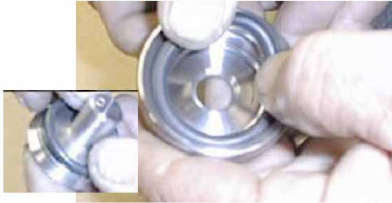
Figure 3-8 Retainer with O-Ring
