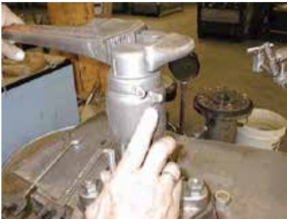
Figure 3-1 Valve Cap Removal
