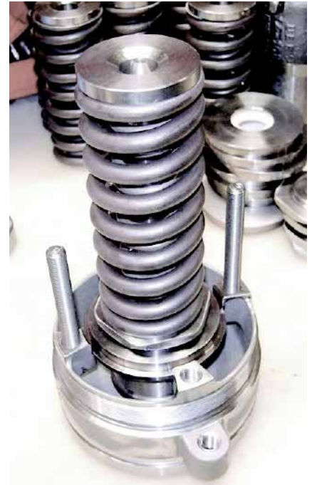
Figure 3-5 Valve After Top Guide Removal
