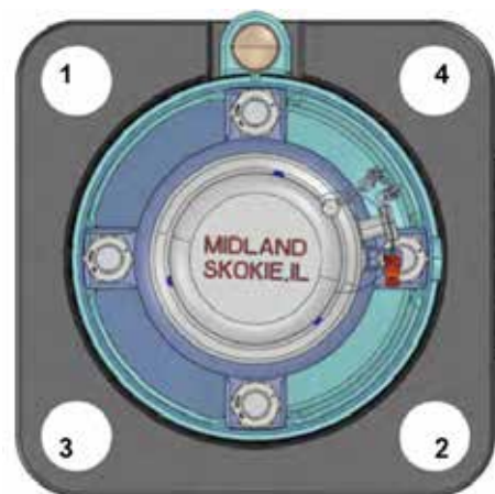
Figure 2-3 Mounting-Nut Tightening Sequence
