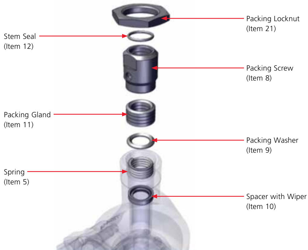
Figure 7-1 Reassembly Steps 7.2.1 through 7.2.7
