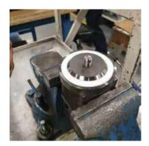
7.2.11.4 Hand tighten the retainer nut (item 20) and use calibrated torque wrench to tighten the retainer nut (item 20) to 35 ft-lbs
