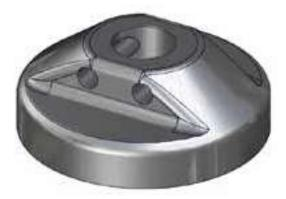
6.1.5 **OUTLET FLANGE**. The surfaces where the O-ring fits, and the flat gasket surfaces must be free of nicks, scratches, and pits. Similarly, the 2" or 3" NPT must be in good condition. It can be cleaned with the standard NPT hand tap. However, a thread gage should be used to be sure the thread is not oversized. The standard hand-tight engagement is 0.436 inches for the thread. The acceptable tolerance is plus or minus one thread. If this tolerance is exceeded, a new part must be obtained.
