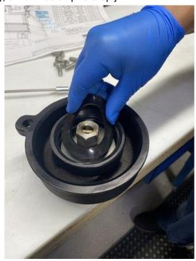
i. Screw the cap onto the top. If the breather vent does not have a check valve, disregard the check valve in the picture.
