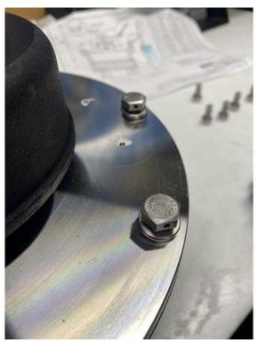
j. Continue hand tightening the bolts in the other holes. These bolts will not have a hole in their head. Use the torque wrench to tighten the bolts to 180 **inch** lbs. (15 ft-lbs.) in a star pattern.
