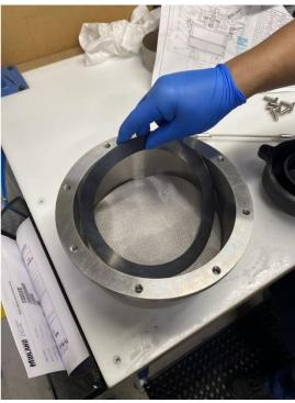
d. Place the filter on top of the filter gasket
