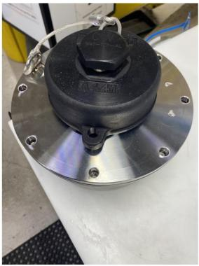
l. Start placing the bolts at the location where the nameplate will go. Make sure to use the bolts with a hole in the head. Put these two bolts next to each other at the nameplate location.
