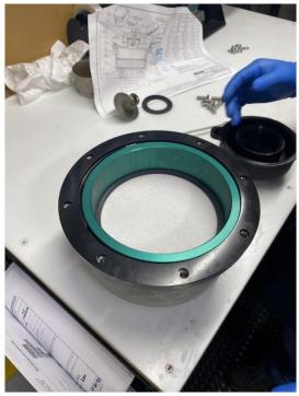
h. If the breather vent has a check valve. Place the top gasket (as shown below) on the check valve assembly, otherwise skip to step j.
