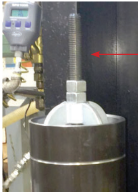
Lubricate valve stem
