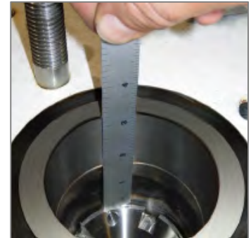
Figure 0-2 Inspect Valve Seat
