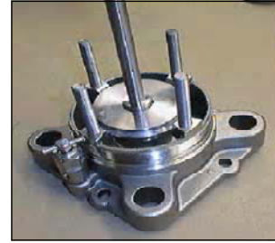
Figure 10 - Valve Stem and Seal Retainer (item 13) and the guide (item 7).
