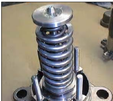
Figure 9 - Valve After Top Guide Removal
