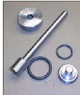
Figure 11 - Retainer, Valve Stem, O-rings and Plug
