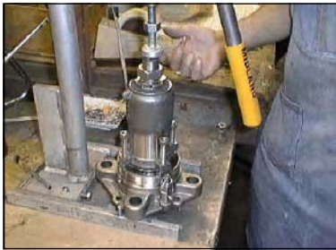
Figure 8 - Clamping for Top Guide Removal
