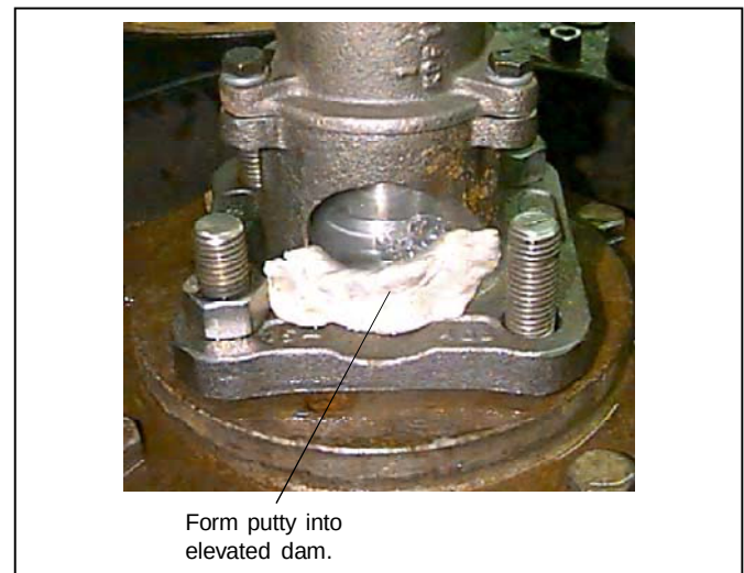
Figure 20 - Blocking Water Drainage With Putty
