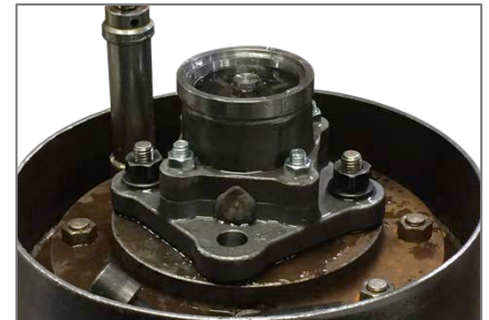
Figure 4-41 Affix Valve to Test Fixture and Seal Drain Holes
