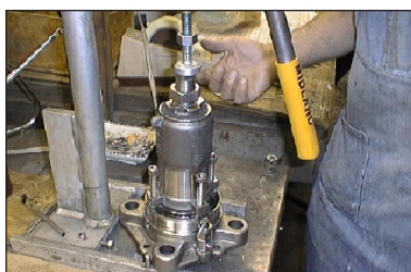
Figure 8 - Clamping for Top Guide Removal
