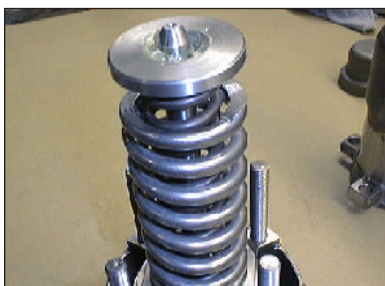
Figure 9 - Valve After Top Guide Removal
