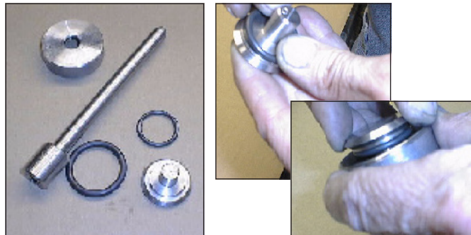
Figure 11 - Retainer, Valve Stem, O-rings and Plug
