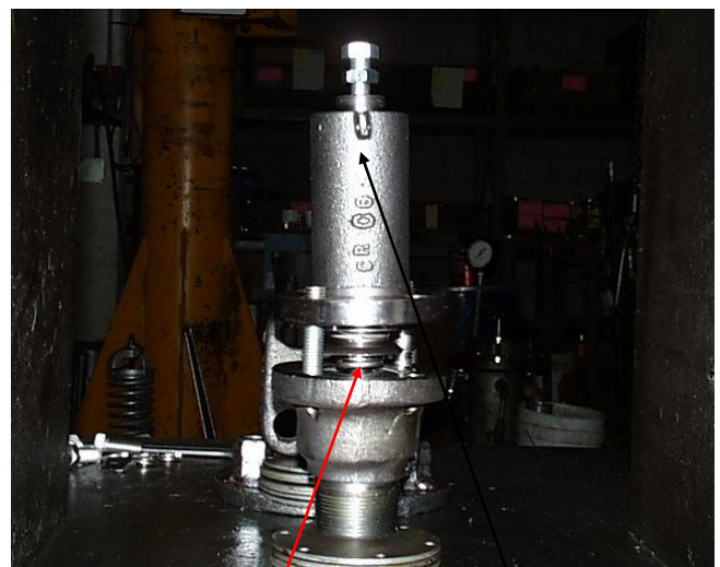
Also, make sure the tip shown in the picture is facing opposite the square flange of body assembly. Indicated here with arrows.
