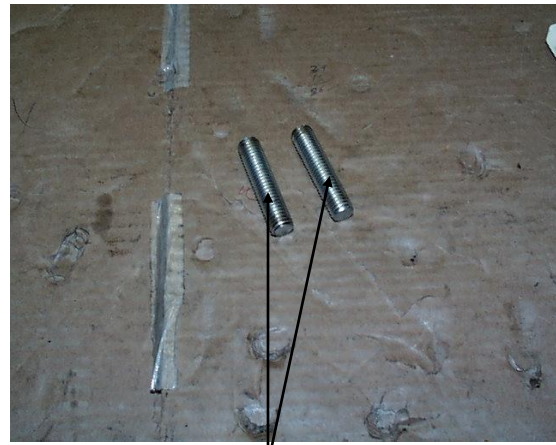
Studs that will help guide the top guide subassembly when pressed.
