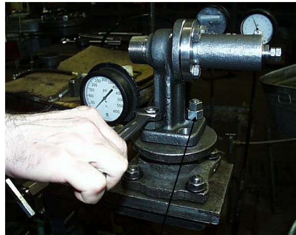
You may use two larger nuts as spacers, as shown.
