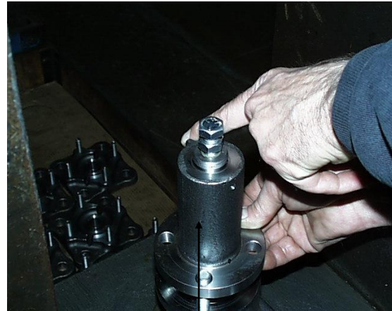
Place the top guide assembly as shown.
