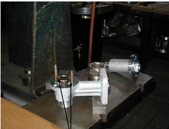
Screw in the studs that will help you guide the top guide assembly.
