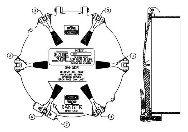
Step 1: Open / Disengage cams (1) and (2), followed by cams (3), and (4)
