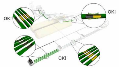
When you replace non-conductive piping on a station with conductive piping you increase the electrostatic safety, even if only a part of the piping system is conductive.
