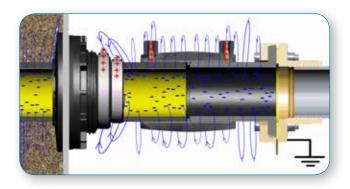
The static charges in the pipe create an electrostatic field and conductive objects in the field will get an induced charge.
