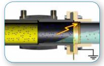
Between negatively charged pipe and grounded conductor.
