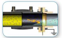
Between negatively charged pipe and positively charged fuel.
