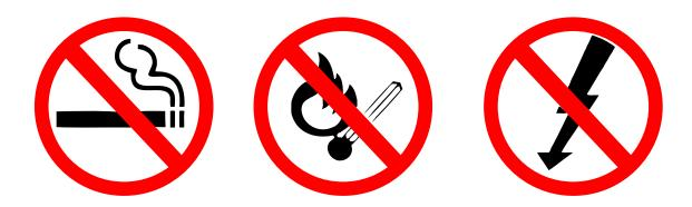
Fire at the filling station is something that needs to be prevented. The risk of a flammable atmosphere occurring is always present where fuel is handled. Just as smoking or open flames are not allowed in the station area, any other possible ignition sources must be eliminated. This includes discharges from static electricity on objects or people.
