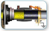
Discharge between two unbonded conductive objects.
