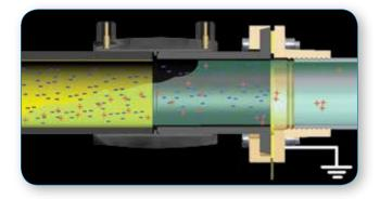
Static electricity is generated when a low conductivity fuel flows in a non-conductive pipe. The fuel will be positively-charged and the pipe wall negatively-charged.
