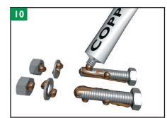
Lubricate the bolts, washers and nuts with copper paste, ceramic paste or MoS2.
