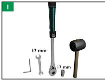
You need: hex key, wrench n:o 17, torque wrench (20-47 Nm) with socket n:o 17 and a rubber mallet.
