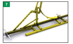
Make sure the pipe rests on the roller castor and between the two heels on the back of the bending tool.
