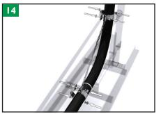
Mount the bolts, washers and nuts with the metal band directly under the bolts.
