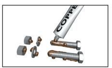
Lubricate stainless steel bolts, washers and nuts with copper paste, ceramic paste or MoS2.
