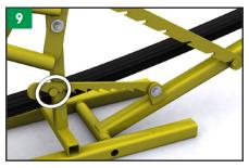
When the locking device clicks into the first notch, release the handle.
