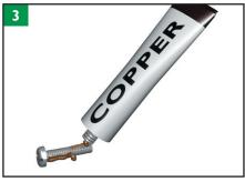
Lubricate the smaller mounting screw using copper paste, ceramic paste or MoS2.
