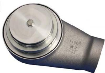
The T195SV Vapor Recovery Vent Mounts using a spanner nut and seal to the manhole plate outside the existing TTMA bolt pattern. This mounting style no longer limits how the vent is mounted. Just angle the vent as needed.
