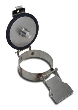
The LJ 10" is a Pressure Relieving Fill Cover unit. The spring loaded fill cap is designed to eliminate flutter during emergency pressure release and to provide a positive seal under normal operating conditions. The LJ cover is equipped with a 3" high weld ring to provide a low profile. This unit is available in either steel or stainless steel material.
