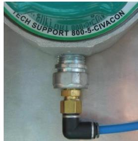
ASA-1 Pressure Switch mounted in ROM Overfill Socket
