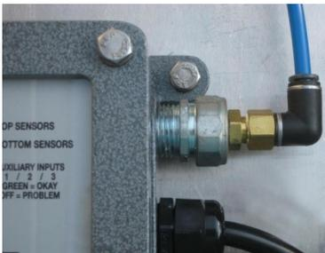
ASA-1 Pressure Switch mounted in ROM Monitor
