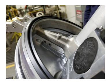
If after installing PN 13226 Fill Opening Gasket, leakage occurs between the Cover and 7700N PAF vent, see troubleshooting steps below. Note: There is no adjustment on the ALVN Manhole Assembly to resolve this issue.
