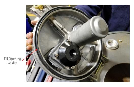
2. Remove existing gasket (you can use a small screw driver to assist with removal. Use caution to avoid scratching the gasket groove).
