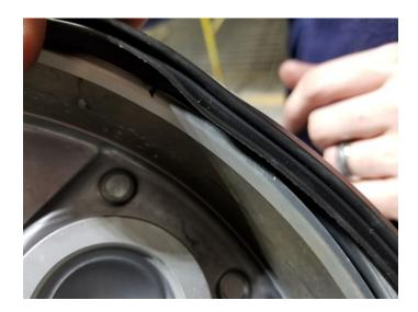
4. Install 4 locations equally spaced around the diameter of the gasket to prevent over-stretching. Finish completely installing the gasket one section at a time.
