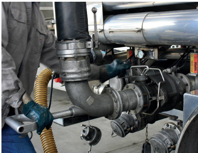
Clearly identified loading arms and driver attention to attaching the right arm to the proper compartment are key to preventing dangerous mis-match mistakes during loading
