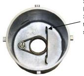
Sensor Tube Retaining Spring. Squeeze ends together to adjust sensor height.
