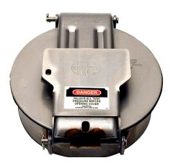
The LJ 10" is a Pressure Relieving Fill Cover unit. The spring loaded fill cap is designed to eliminate flutter during emergency pressure release and to provide a positive seal under normal operating conditions. The LJ cover is equipped with a 3" high weld ring to provide a low profile. This unit is available in either steel or stainless steel material.
