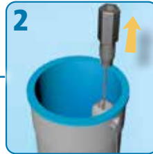
Lift float with cable to simulate fill
