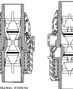
OPERATING POSITION: POPPETS OPEN, INTERLOCK ENGAGED, COUPLING IN CONTACT WITH FORCE RAMPS.
