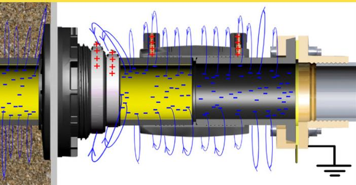
The static charges in the pipe create an electrostatic field and conductive objects in the field will get an induced charge.
