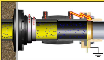
Discharge between two unbonded conductive objects.
