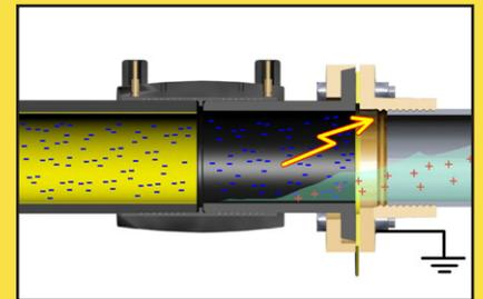
Between negatively charged pipe and grounded conductor.
