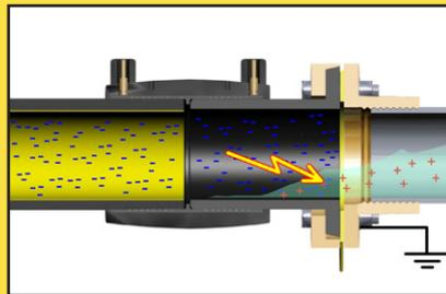
Between negatively charged pipe and positively charged fuel.
