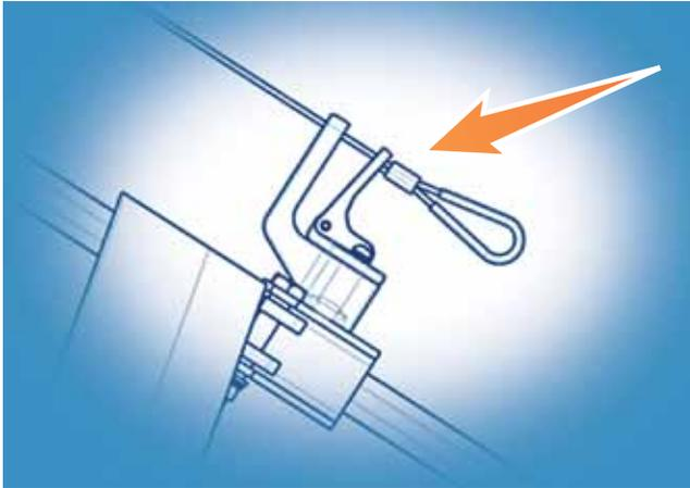
The Cable Release mounting option, which is available with a cable up to 69 inches long, prevents material collection within the brake-release handle.
