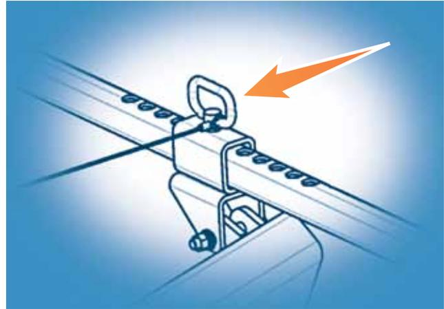
The Manual Release mounting option relies on a pin to lock the loading arm in place when dealing with heavy loads.
