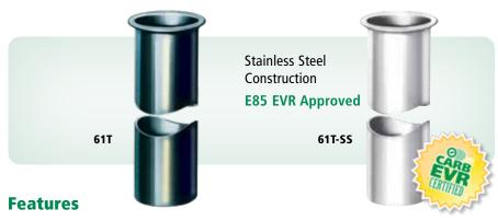
.062" Thick Drop Tube Walls – deter denting and damage to the tube upon installation or removal for long service life.  Various Lengths and Diameters – accommodate a variety of tank diameters and fill riser pipe sizes.
