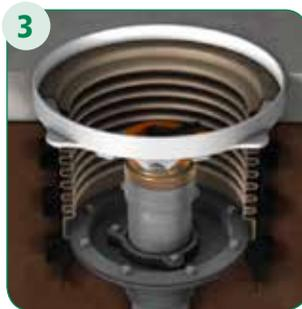
3 Replace Bellows, Reinstall Upper and Lower Rings
