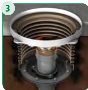
Replace Bellows, Reinstall Upper and Lower Rings
