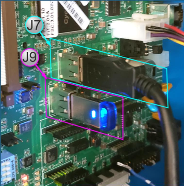
There are two (2) internal USB ports on the PV100 Main Board.
