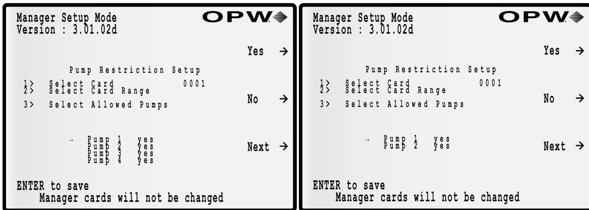
Pump Restrictions - 4 Pump Setup & 2 Pump Setup
