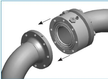
**Step 3:** Once the now-detached arm has been secured and put out of the way, remove the three (3) O-rings and two (2) O-ring spacers. Inspect and clean all machined surfaces to ensure that there are no nicks, scratches or burrs.
