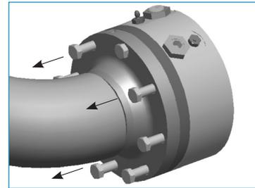
**Step 6:** Align flange with body and press surfaces together. Thread flange bolts with Nord-Lok™ washers into tail and torque to amount shown on chart. Nord-Lok™ washers come as an assembly bonded together from the factory. It is important that the correct orientation be preserved for proper function.
