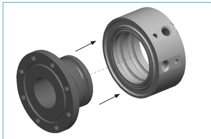
**Step 5:** Carefully align swivel tail and insert into body.
