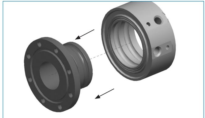
**Step 3:** After all balls have been removed, carefully remove swivel tail from swivel body.
