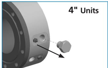
**Step 2:** Remove ball bearings via ball port in swivel body. NOTE: Non-flammable solvent may be used to help loosen lubricant and allow for easier ball removal.
