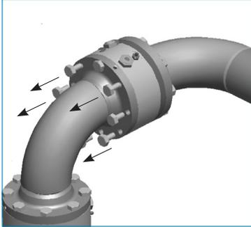
**Step 2:** Remove all split flange bolts on the side of the swivel attached to the free-moving end. With the bolts loosened, support this side of the loading arm along with any other parts attached to it that might move freely when the bolts are removed. Remove bolts, starting with lowest on flange, leaving top bolts for last. Be careful not to damage sealing flange module face and bolts.
