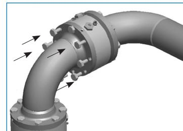
**Step 8:** Bolt sealing flange to body using bolts and Nord-Lok™ washers. Torque to amount shown on chart below.
