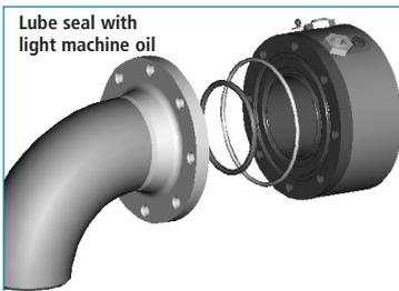
Lube seal with light machine oil
