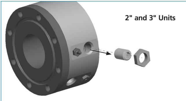
**Step 1:** Remove bearing plug bolts to access respective ball race.
