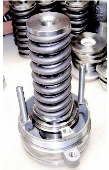
Figure 3-5 Valve After Top Guide Removal
