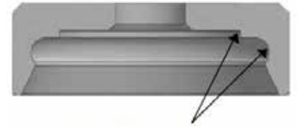
Check Surfaces of Grooves for Nicks, Gouges and Corrosion
