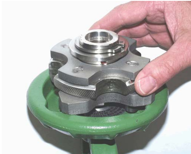
Coupler not properly engaged
