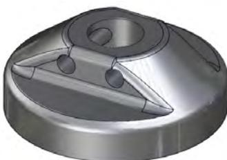
Figure 6-3 Gasket Retainer
