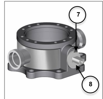
Figure 4-20 Install Stop Plate
