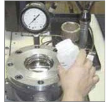
Figure 4-34 Immerse Seal for Leak Test
