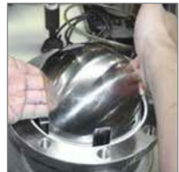
Figure 4-26 Install Valve Ball
