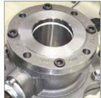
Figure 4-32 Tighten Cap Screws
