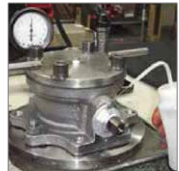
Figure 4-35 Valve Stem Leak Test
