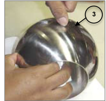
Figure 4-14 Check Scratch Severity
