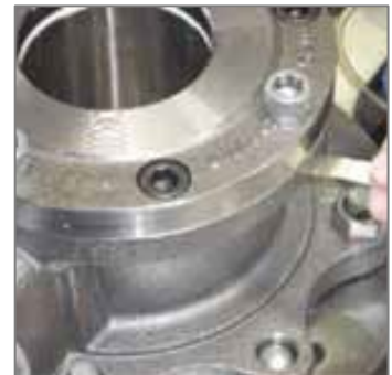
Figure 4-33 Check Cap-to-Body Contacts
