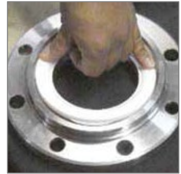
Figure 4-27 Install Ball Seal
