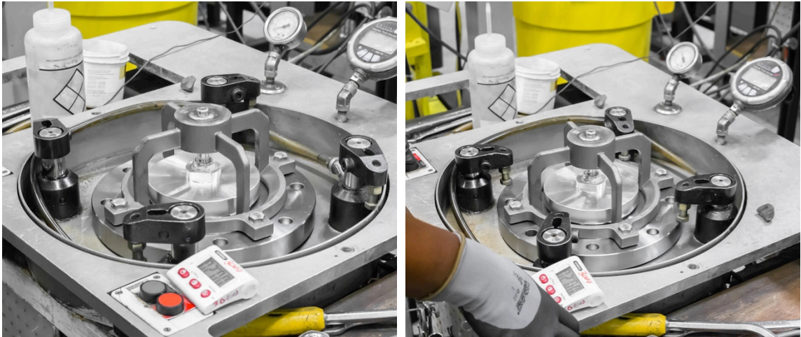
Figure 7-1 Affix Valve to Test Fixture
