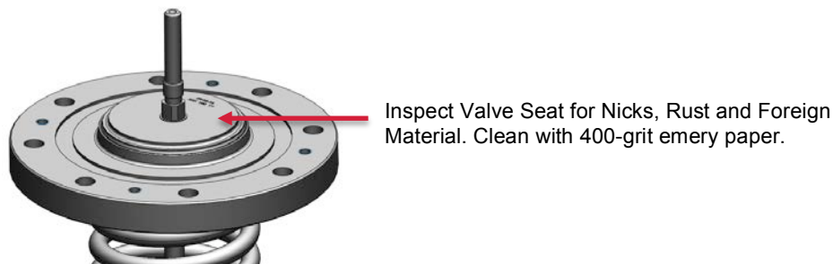
Figure 9-6 Inspect Seat Surfaces
