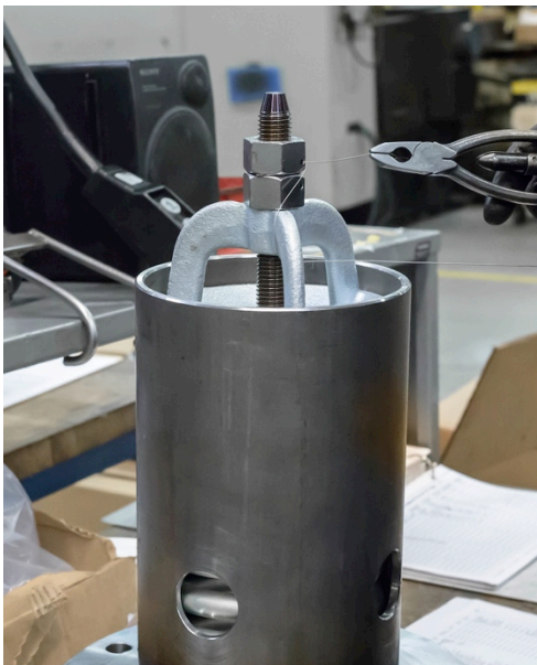
Figure 8-9 Apply Seal Wire
