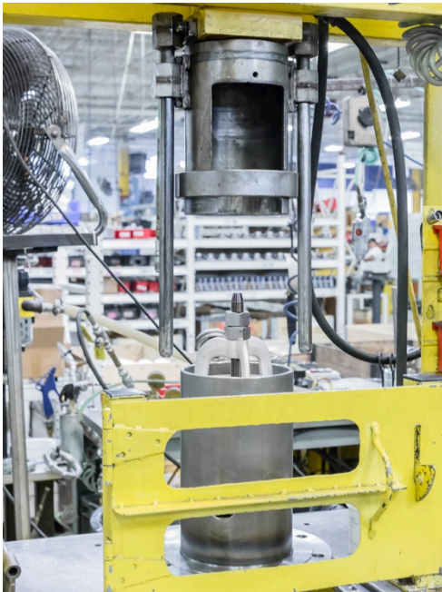
Figure 8-6 Release Spring Compressor
