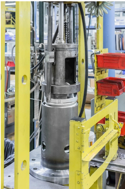
Figure 8-4 Compress Valve Spring
