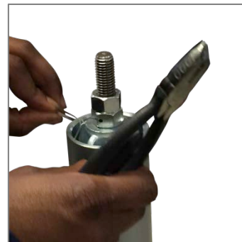
Figure 4-50 Install Seal Wire
