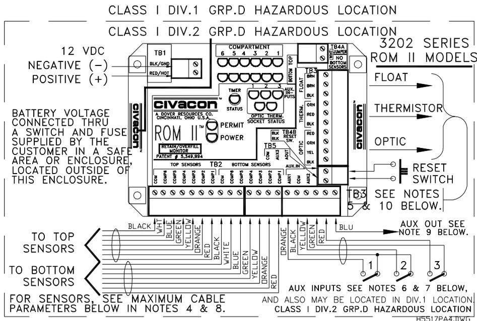
**FIGURE 5 - POWER AND INTRINSICALLY SAFE WIRING
