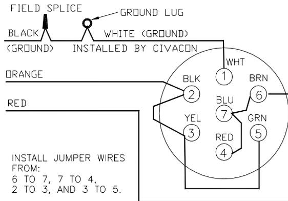
**FIGURE 7 - THERMISTOR VIEWED FROM WIRE CONNECTION SIDE**
