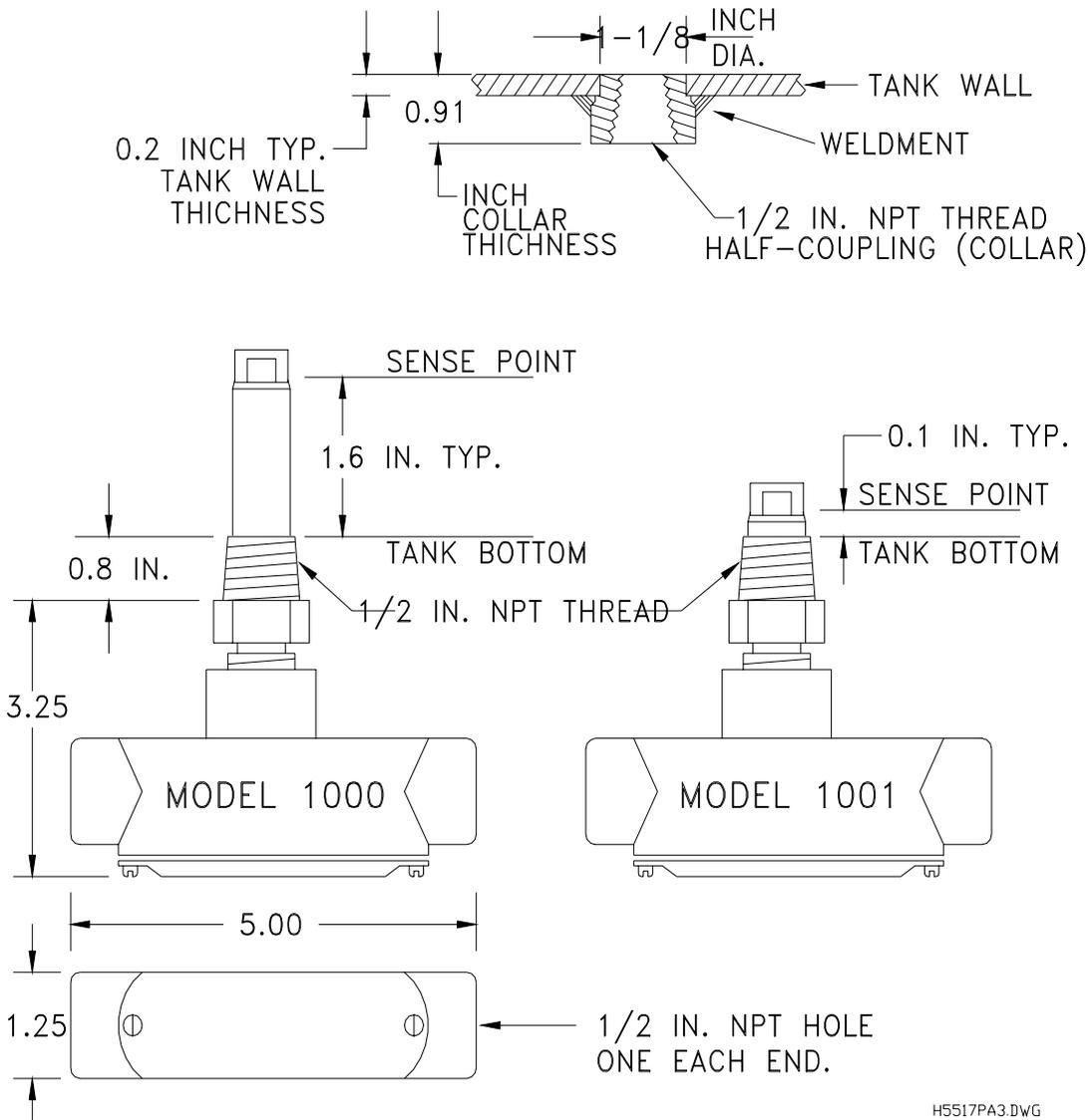
**FIGURE 4 - RETAIN SENSOR DIMENSIONS**
