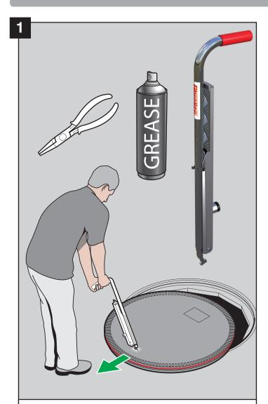
To replace the existing gasket, you will require an FL7A lifting handle, a pair of needle nose pliers and a can of white lithium spray grease. To begin, remove the cover from the frame using the FL7A lifting handle.
